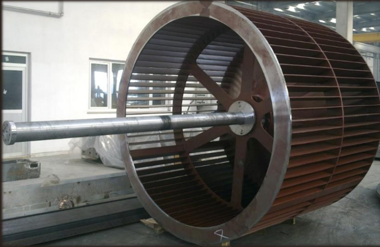
SEPARATOR ROTOR PFEIFFER SLS 4000B K.MARAŞ CEMENT PLANT K.MARAŞ / TURKEY 2013/2014
